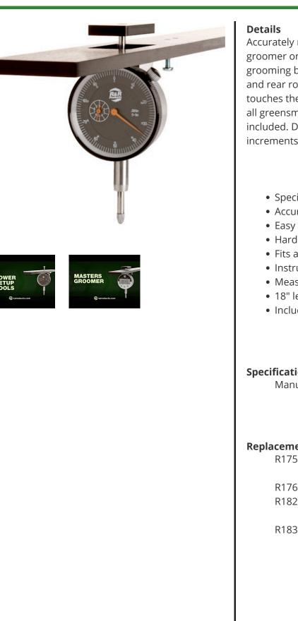
Accurately measures desired grooming depth of groomer or verticut units. Easy to use. Rotate the grooming blade facing down, place the bar on front and rear rollers then push the measuring rod until it touches the blades. Hard anodized aluminum. Fits all greensmowers. Instructions and conversion included. Displays measurements in .001" increments. 18" length.
