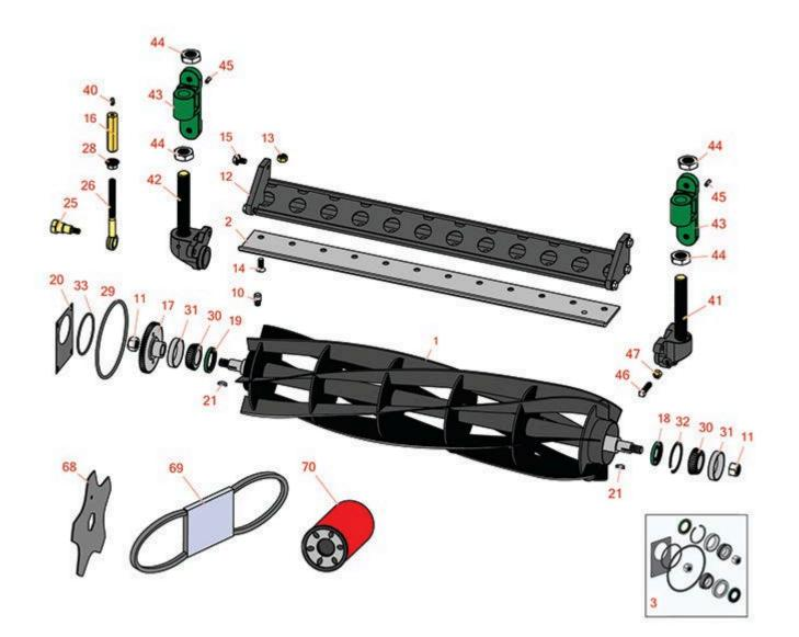
ESP Cutting Unit Model 303, 305, 756, 856, 3325 & 3365 Reel & Bedknife
