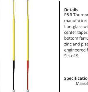
R&R Tournament Tapered Flagsticks are manufactured from solid color-impregnated fiberglass which will not chip or fade. 3/4" diameter center tapers to 1/2" on top and bottom. Top and bottom ferrules manufactured with durable cast zinc and plated for extended wear. Precision engineered fit with either plastic or aluminum cups.
